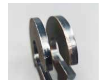
Carbon steel bright surface cutting
