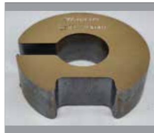
20mm carbon steel cutting
