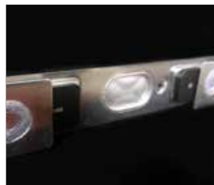
Explosion-proof valve welding
