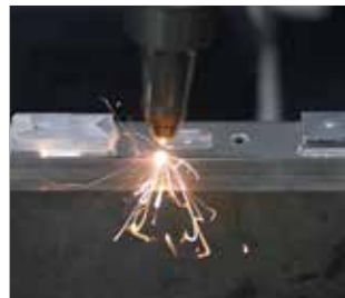
Lithium battery welding
